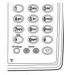
Adjust the volume of the base speaker by pressing the **volume** keys on the base. Press  $\blacktriangle$  for louder or  $\blacktriangledown$ for softer.
