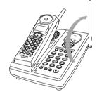
5 Connect the telephone line cord to the TEL LINE jack and a telephone outlet once the handset is fully charged.
