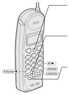
1 Press and hold <u>mem</u> for 2 seconds. The display shows the memory screen and any saved name/number.
