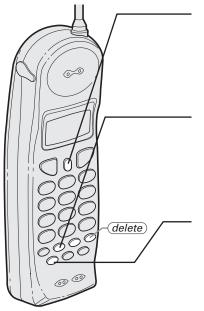
1 Press and hold <u>mem</u> for 2 seconds. The display shows the memory screen and any saved name/number.
