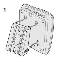
1 Snap the wall mount adapter into the notches on the base.
