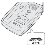
Check the LED display to see if the answering machine is on or off. If the LED display is on, the unit is on and ready to take messages. If the LED display is off, it will not take messages.
