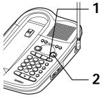
During the conversation from the handset. Press and hold *voice memo* on the base. The unit begins recording and the LED blinks. Both parties can hear tones every 15 seconds.
