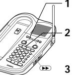
On the base, press and hold *pin* button until a tone sounds, and the LED displays 30.
