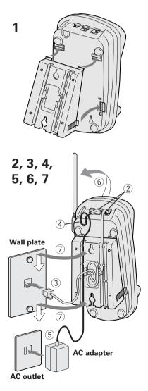
**1** Snap the wall mount adapter into the notches on the base.
