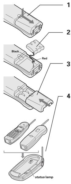
Press and slide the battery compartment cover toward the bottom of the unit.
