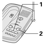
During the conversation from the handset, press and hold *voice memo* on the base. The unit begins recording and the LED blinks. Both parties can hear tones every 15 seconds.
