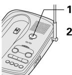
1 Press <u>speaker</u> on the base to join the 3-way conversation.
