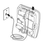
6. Align the mounting slots on the base with the mounting screws on the wall. Push in and down until the phone is firmly seated.
