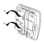
On the base, pull the handset retainer out of the slot. Rotate clockwise 180°.
