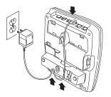
Plug one end of the short telephone cord into the *TEL LINE 1/2* jack on the back of the base. Plug the other end into a standard telephone jack.
