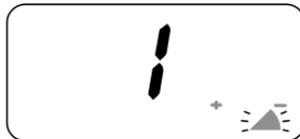
When the batteries in the unit are low, the unit will go into a Battery Low/Sleep Mode. The Scan Mode, Transmit, Transmit Call Tone Mode, CTCSS Tone Setting Mode, and Vibration are disabled. Replace the batteries immediately to continue using the radio.
