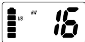
When the battery is nearly discharged, the battery indicator appears as follows:
