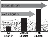
Setting the squelch level higher filters out noise and lets only actual radio transmissions through.
