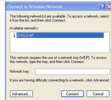
3. If the chosen network requires WEP encryption, you will have to enter the WEP key for your network in the **Network key** field as shown in the screen below.
