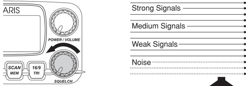
Turn **SQUELCH** back clockwise until the hiss stops. Now the “Squelch Gate” allows only strong signals through.
