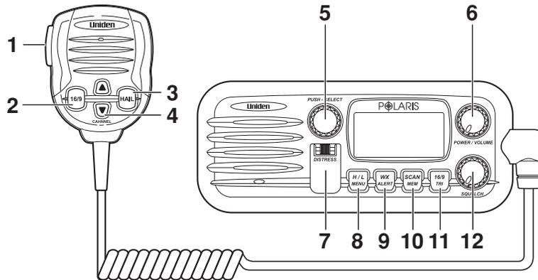
1. **PTT Switch** - Press to transmit and release to receive.
