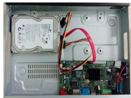
Connect HDD power lines and data cable
