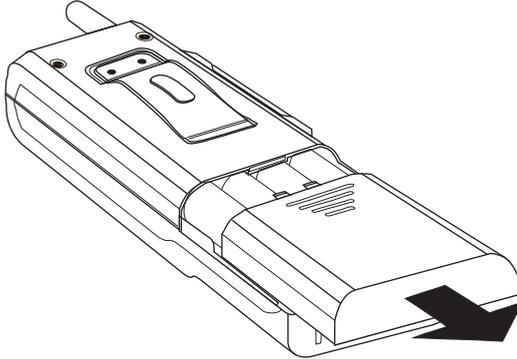
2. Insert 10 nickel cadmium batteries in the compartment.
