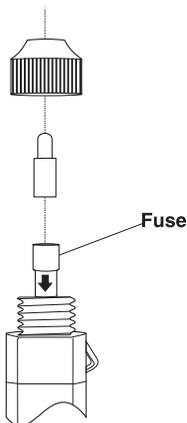
2. Remove the fuse and replace it with the same type.
