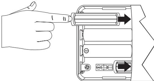
3. Insert 8 alkaline batteries into the compartment as shown.
