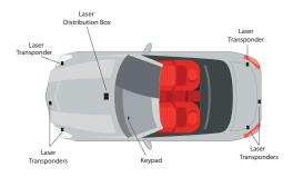
Connect the Laser Distribution Box to the RJ11 port on the R4w or R8w. Connect the Keypad to the RJ11 port on the Power Adapter.
