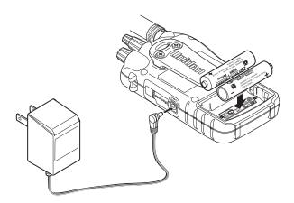
You can power your scanner using two alkaline, or rechargeable AA batteries.
