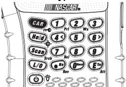
Your scanner's keys have various functions labeled on the key tops and below the keys. To select the function labeled on a key, simply press the key. To select the function labeled below a key, hold down Func on the left side of the scanner then press the key.
