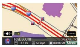
Heading up view (2D): (default) The direction you are currently going is always at the top of the screen. The car icon points up, and the map rotates as you change direction. The COMPASS icon's red needle rotates to point north.
