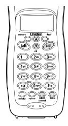
1) Press *cid*. 2) Press (delete). 3) Press ▲ or ▼ to select "∀es" or "No". 4) Press (select/channel) or (delete). When the pointer is at " $\forall e \equiv$ ": A tone sounds and all stored Caller ID messages are deleted. When the pointer is at "No":
