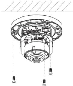
4. Adjust surveillance angle. Loosen one tilting adjustment screw and adjust as needed. Tighten the screw.
