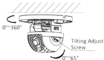
5. Hold the black liner to adjust the pan position.
