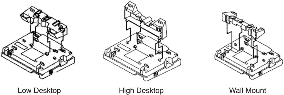
**Figure 2-1 Footstand Mounting**
