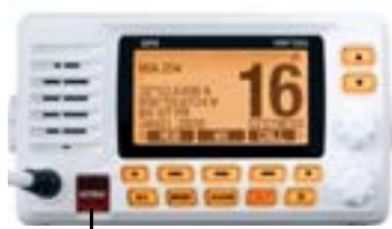
Lift the red cover and press the DISTRESS button underneath
