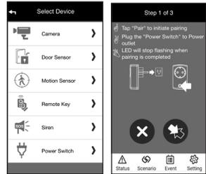
2. Follow the screen instructions for pairing the sensor. After pairing is complete, plug a light fixture into the sensor. Tap **△** to display the sensor Status screen.
