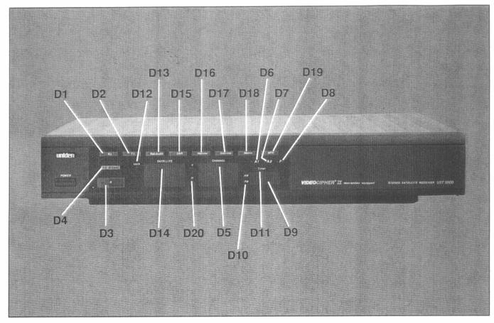
**D1. Ku LED** - Lights when Ku-band reception is selected. Turns off when C-band mode is selected.
