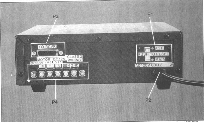
P1. Circuit Breakers - If unit fails to light up when the power button is pressed, try pressing the MAIN circuit breaker. If unit lights up but fails to move the antenna, try pressing the ACT circuit breaker.
