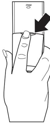
2. Slide the battery compartment cover down.
