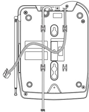
5. Plug the telephone cord into the modular jack on the wall.
