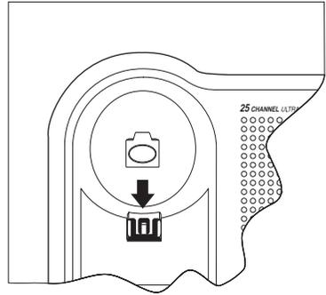
4. Push down on the Handset Retainer until it snaps into place.
