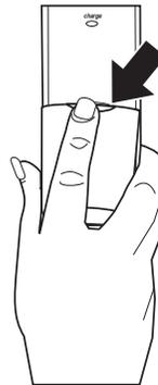
2. Slide the battery compartment cover down.
