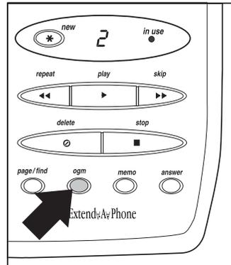
2. Do not get closer than twelve inches from the microphone, and speak clearly while recording your message. When you are finished recording, release **ogm**.
