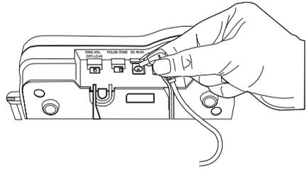
4. Place the AC Adapter cord inside the molded channel.
