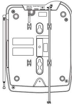
4. Plug the AC Adapter into the Base Unit.
