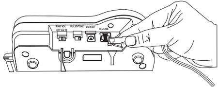
2. Place the telephone cord inside the molded channel on the bottom of the Base Unit.
