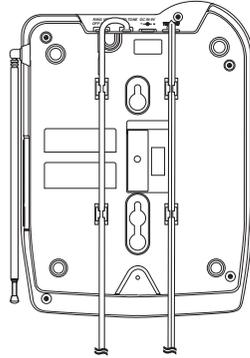
6. Place the Base Unit on the screws and push down until it's firmly seated.
