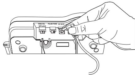
5. Place the AC Adapter cord inside the molded channel.
