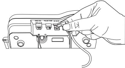
4. Place the AC Adapter cord around the strain relief.
