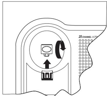
3. Put the retainer back into its slot on the Base Unit.
