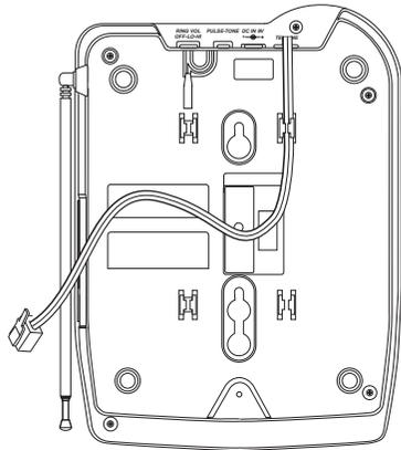
3. Plug the AC Adapter into the Base Unit.
