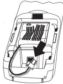
4. Place the battery pack inside the battery compartment, and slide the battery cover back on.
