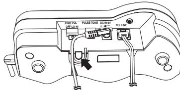
5. Plug the other end of the cord into the telephone jack on the wall.
