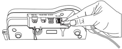
3. Place the cord inside the molded channel on the bottom of the Base Unit.
