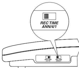
**Note:** If the **REC TIME/ANN/4/1** switch is in the "Announce Only" position, the Message Counter LED displays an **A** when the system is in Standby.
