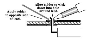
Use a similar soldering technique when installing components in multilayer boards. Note that plate-through vias *do not require soldering* because electrical contact is already established between layers by the plate-through itself.
