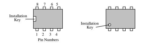
□ Align the key on the IC body so it corresponds with the key of socket U1. Loosely insert the pins of the socket into U1. All 8 pins should fit freely into the socket openings. If not, straighten the IC pins until they do. Using firm and steady pressure, fully seat the IC into the socket.
