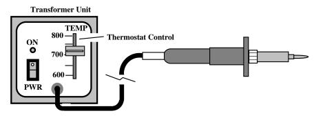
**Mini-Irons:** With the advent of surface-mount technology and increased miniaturization, a smaller version of the conventional soldering iron has gained popularity. Light-weight "mini-irons" (or soldering pencils) outfitted with ultra-fine tips reach into tight spots where other irons can't reach. Mini-irons are available in both unregulated and thermostatically-controlled models.
