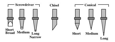
Some manufacturers offer special variations such as the "bent conical tip" or "micropoint tip" for special applications. Also, for slightly better heat transfer, some narrow screwdriver tips may be used interchangeably with the longer conical tips.
