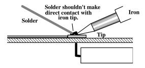
Solder should melt, flow, and wet the surface of the lead and pad to form a bright smooth connection. Rocking the iron slightly as solder flows will promote better solder distribution around the connection.
