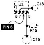
□ □ 10. Trim the exposed wire from one end the insulated jumper wire to about 1/16". Solder this end of the insulated jumper wire to pin 6. <u>Be</u> <u>very careful not to bridge adjacent IC socket pins!</u>
