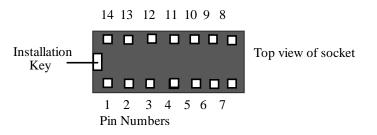
□□ 5. Install and solder the 14-pin IC socket at location U1. Observe that the key aligns with the legend outline on the PC board.
