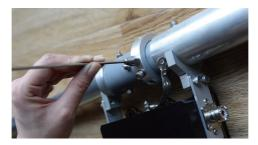
\*Please make sure that each main rod is connected and fastened well; otherwise the overall strength of the antenna shall be affected.
