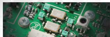
3 kHz and 15 kHz Roofing Filter
