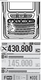
When a local node is found, [X] is lit solid, and the node name and city name appear on the bottom part of the screen.
